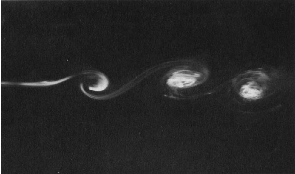
FIGURE 1. Side view of vortex-roll growth and breakdown in mixing layer in 'still air'. High-velocity stream is on upper side. Reynolds number based on length of photograph approximately 10 000.
