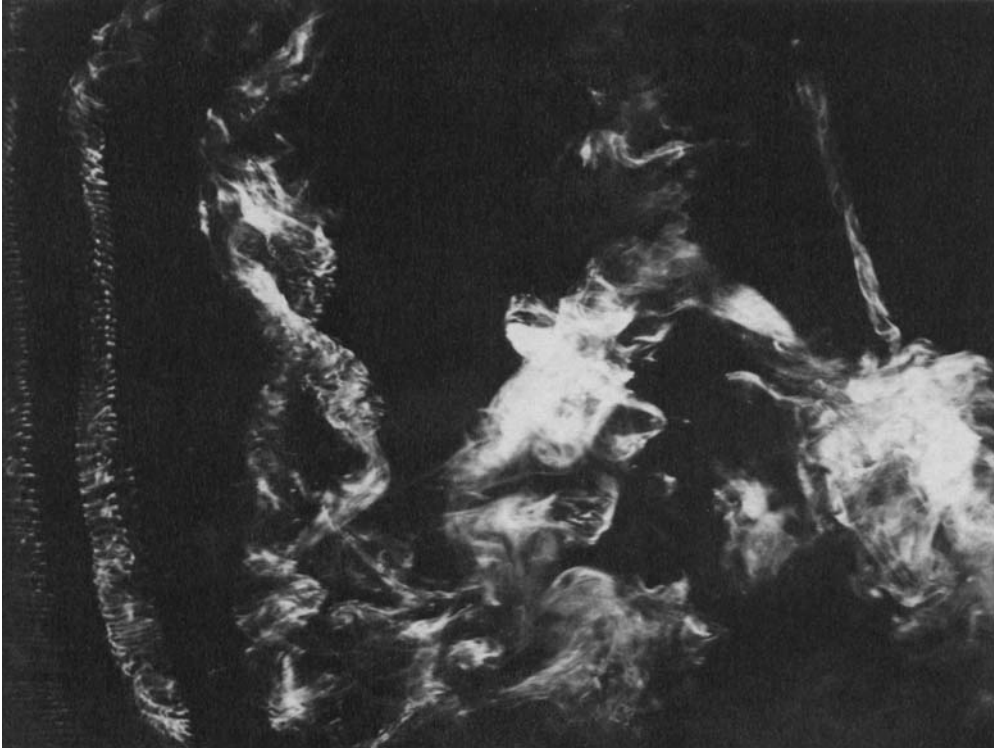
FIGURE 3. Plan view of double-helix vortex pairing. Conditions as in figure 2.
